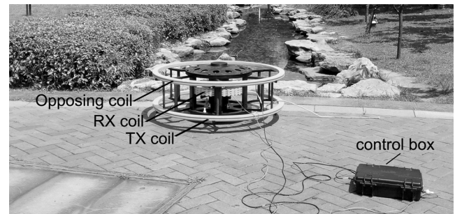
Figure 3. The opposing-coils TEM prototype. The opposing coil and TX coil are 1.2 m in diameter and 10 turns. Distance between the opposing coil and TX coil is 0.3 m. The RX coil is 0.5 m in diameter and 100 turns with an effective area of 19.63 m 2 .
